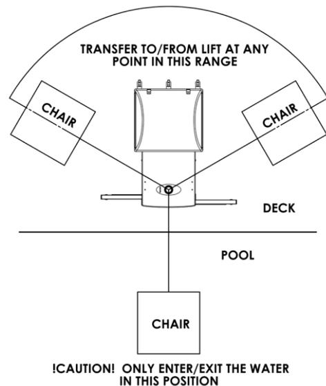
Using the directional buttons on remote return lift chair to a position in the deck loading range. To Exit the Pool or Spa:
