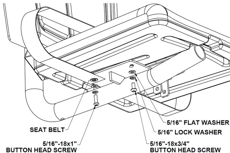
*Note: When attaching the seat belt use 5/16"-18 x 1" as shown below.*
