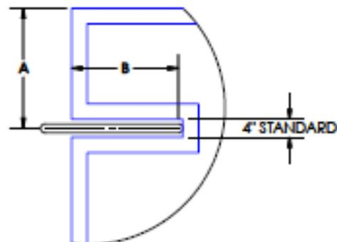
MEASURING RAIL LOCATIONS EDGE OF POOL TO Q OF RAIL
