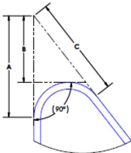
MEASURING ROUNDED CORNERS LESS THAN 90°
