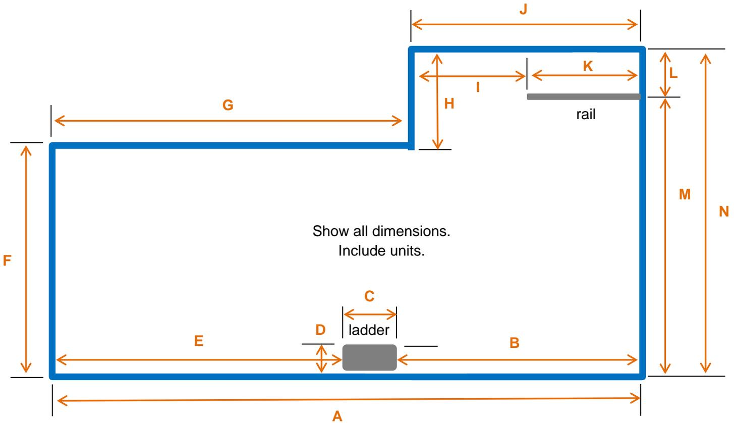
1. Measure all lengths and widths of the pool.
